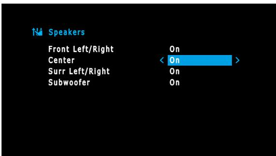
5. Use the Up/Down buttons to select a speaker group and use the Left/Right buttons to select "On" when the speakers are present in the system, or "Off" for positions where no speakers are installed. The Front Left/Right setting is always On and may not be disabled. (Note: The settings in this menu affect the remainder of the speaker-setup process and the availability of various surround-sound modes.)
