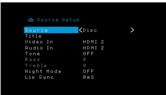
5. Select “Video In” and select the video input connector you want to assign to the source button. Press the OK button. NOTE: If you select an HDMI connector as the video input connector, the audio input connector will automatically change to the same HDMI connector. You cannot use a different audio input connector with an HDMI video input connector.
